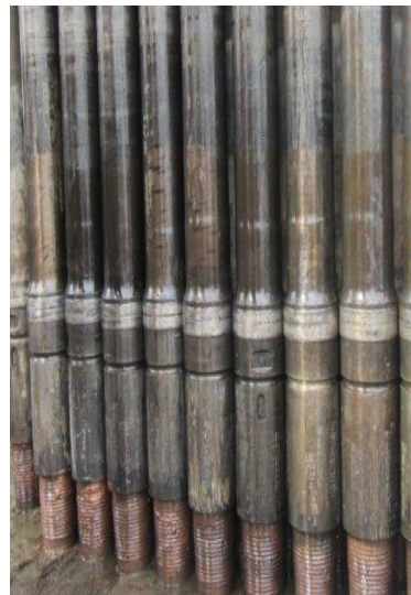
Drillstring after pumping BaraKlean®-926 casing cleaner
