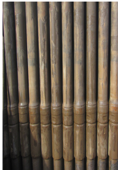
Drillstring before pumping BaraKlean®-926 casing cleaner
