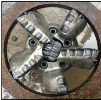
Photo showing minimal cutting structure damage (Dull Grade: 0-0-NO-A-X-I-CT-DTF) after 1 st run of the Crush & Shear hybrid drill bit.
