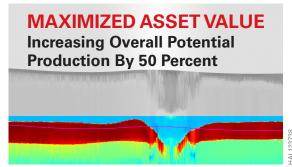
Model illustrating the use of EarthStar™ real-time data to identify and contact a secondary oil-bearing target after entering a large water-bearing zone.
