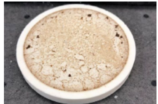
Filter cake removed after a seven-day soaking period with BDF™-442 filter cake breaker. Testing indicated greater than 80 percent return permeability.
