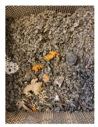
The Vali Tech® filter collected 84 lbs of sponge balls, cement, composite, aluminum, cuttings, and steel swarf debris.
