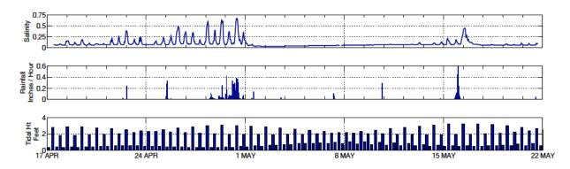
Figure 4. The Salinity sensor on the Hach Hydromet DS5 clearly resolves the small tidally driven salinity differences between Foreman Branch and the Chester River, until the large rain events in late April and mid May reduce the River salinity to nearly zero.
