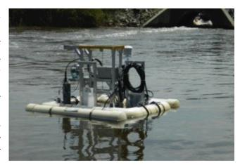
Figure 1. Sea-Bird Coastal / Hach Hydromet Foreman Branch Nutrient and Water Quality monitoring platform located on Chino Farms.
