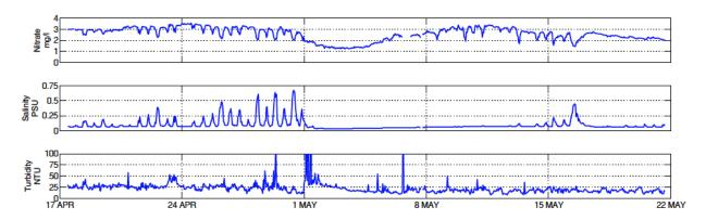
Figure 5. At times of lower flow, Foreman Branch Nitrate concentration varies from around 3 mg/l at low tide (representing flow through the weir) to around 2 mg/l at high tide (influenced by the lower mean Chester R concentration). High post-rain flows dilute the concentrations to around 1 mg/l (but total Nitrate input likely increases due to the larger flows). Turbidity spikes >100 NTU immediately follow the rain event.
