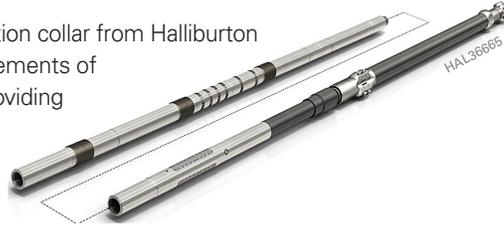
The DrillDOC collar runs with the Sperry Drilling pressure-while-drilling (PWD) tool. Measurements from the PWD tool compensate for pressure and temperature changes downhole, and help ensure the accuracy of the DrillDOC collar's measurements through the full range of temperatures and pressures in all well conditions.
