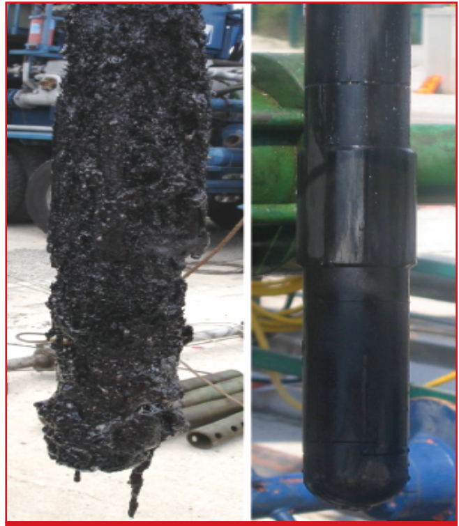
Figure 1 - Bottomhole assembly fouled with asphaltene (left) prior to DuraKleen service and (right) following the service.
